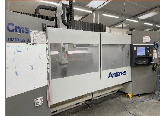
Machine d'usinage 5 axes 2500mm x 1500mm x 1200mm
